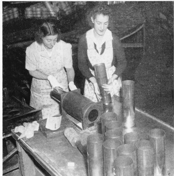
Margaret Whalen is testing the cases in a model gun breech to see that they fit right. Right beside her, Mary Greguoli looks for any possible defects. The finished shell cases must pass rigid inspection.
