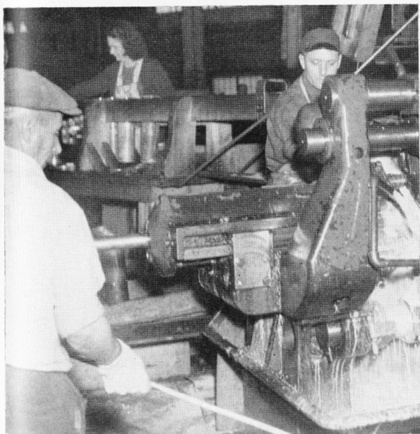
Clemento Vilardo and John Zampino are operating a Gridley machine which shaves down the base and flange so they will be the exact size to fit the breech of the gun for which it is being made.
