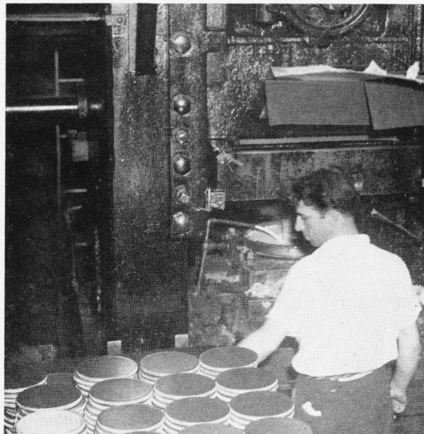
The circular disks of metal are passed along to the next operator, in this instance Albert Colaninno. His machine will transform the disk into a heavy cup-shaped object, something which really looks as if it could be developed into a full size, dangerous and powerful shell for use in our fight to eliminate the enemy.
